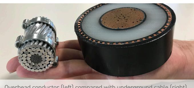
the conductor. Underground cables require an outer protective jacket, shielding and insulation to keep the conductor cool.
