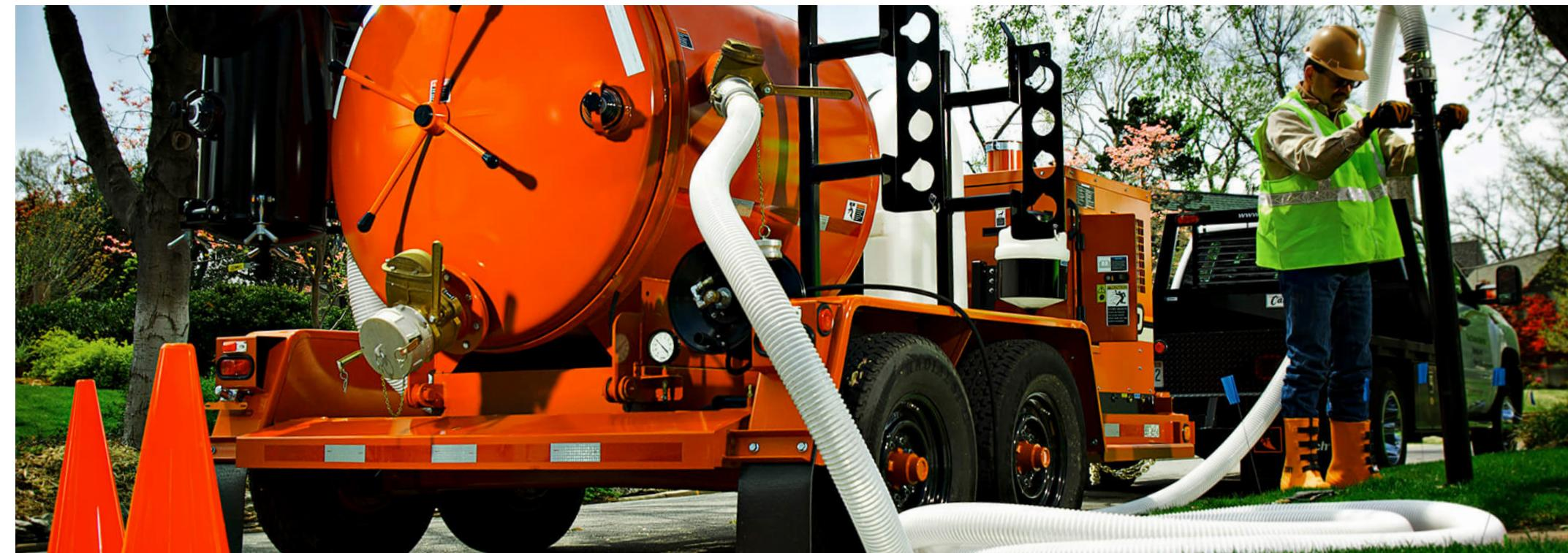
**Hydro Excavation:** Crews use hydro excavation (hydrovac) in areas where many underground utilities are located near each other. This process involves using pressurized water to break down soil to expose underground utilities. Afterward, crews backfill the area. The process helps prevent damage to underground infrastructure while gathering important information.
