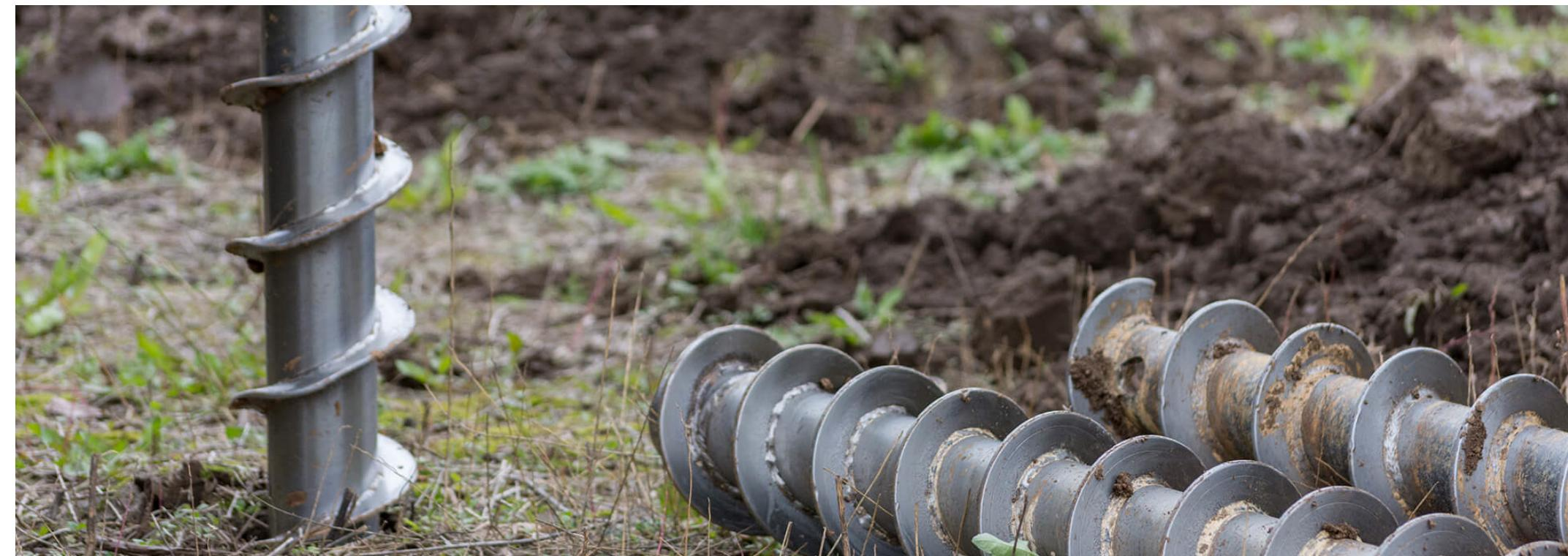
**Soil Borings:** Field crews use a drill to bring up soil samples and then backfill the holes. Testing the core samples helps determine soil conditions in the area. Soil conditions and types can affect structure location and foundation design.
