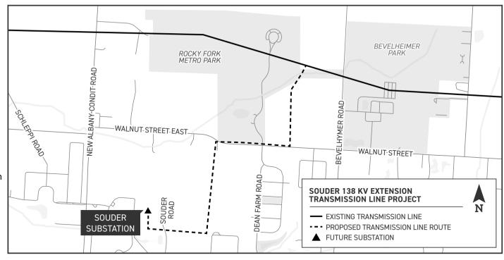
AEP Ohio representatives have filed a Letter of Notification with the Ohio Power Siting Board (OPSB) as Souder 138 kV Extension Transmission Line Project, Public Utilities Commission of Ohio Case No. 25-0704-EL-BLN. The Letter of Notification to construct, operate and maintain this facility awaits OPSB review. If approved, company officials expect construction to begin this fall and conclude summer 2026.
